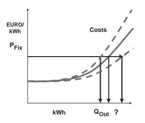
Fig. 1. How a feed-in tariff works.
