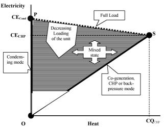
The full-load line PS slopes down. The downward slope indicates the loss in power that occurs by extracting the steam from the turbine above condensing conditions (the latter being near vacuum pressure and near ambient temperature). The higher the pressure and the temperature of the heat extraction are the more power that is lost for every Joule of
