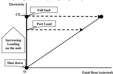
Figure 1 Thermal power generation always brings along the output of fatal heat
