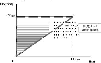
Figure 9 CHP design and scale should cover most of the heat loads while maintaining the maximum quality (power-to-heat ratio)
