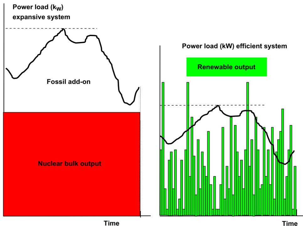
Fig. 3. Fossil add-on to nuclear bulk output versus the fluctuating renewable power.
