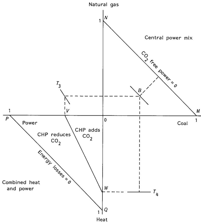
Figure 5. Reducing or increasing CO<sub>2</sub> by CHP, given a particular central power mix (point B).
