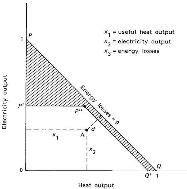
**Figure 1.** Energy conversion in a CHP process.<sup>a</sup>
