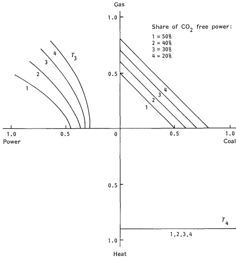
Figure 7. Transformation curves  $T_3$  and  $T_4$  for various central power mixes.
