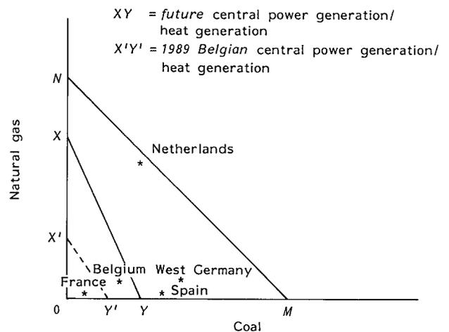
**Figure 4.** Reducing or increasing CO<sub>2</sub> by CHP in five countries, given a particular CHP process (electric efficiency = 30%; heat efficiency = 50%) and 1989 Belgian central power mix.
