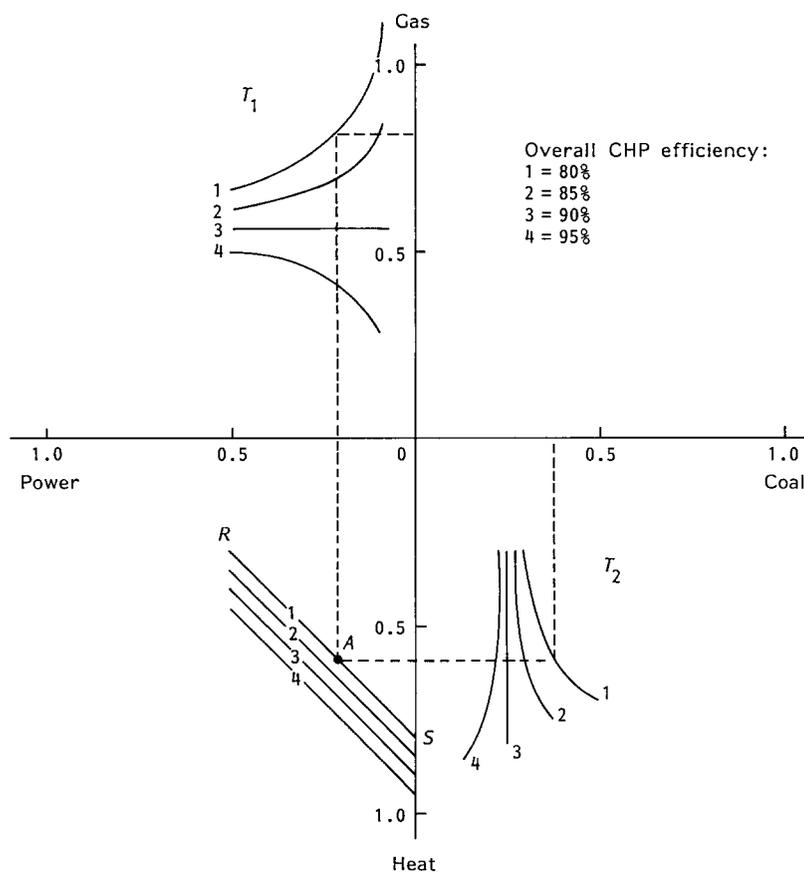
**Figure 6.** Transformation curves  $T_1$  and  $T_2$  for several overall efficiencies of the CHP process.
