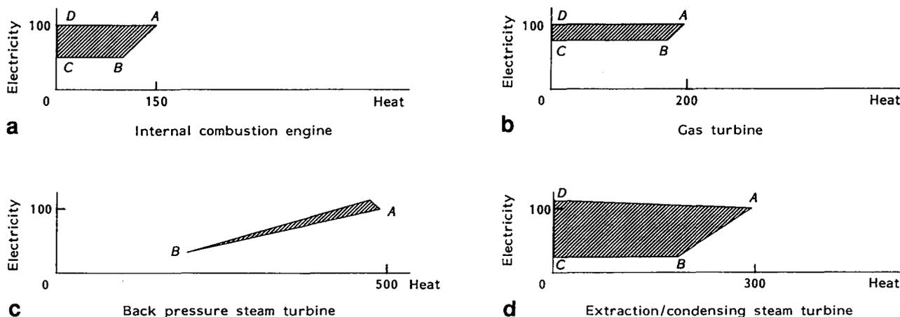
**Figure 5.** Production possibility sets of CHP process (capacities shown relative to maximum power output = 100).
