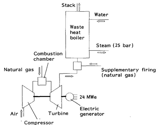
Figure 7. Gas turbine with supplementary firing.
