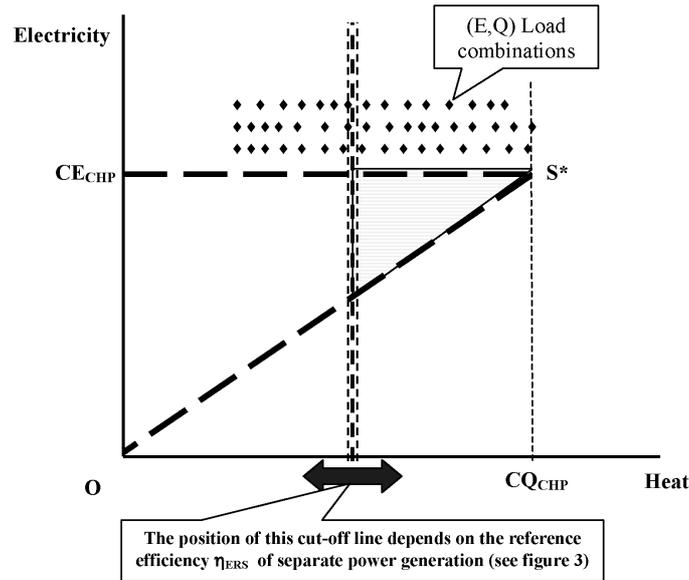
Normally the plant owner will want to operate the unit at maximum load, generating  $CE_{\text{CHP}}$  along the top line  $CE_{\text{CHP}} - S^*$  of the possibility set. In addition, he will have to buy some make-up power at the grid (shown by the vertical distance from the load point to line  $CE_{\text{CHP}} - S^*$ ). He also will have to waste<sup>2</sup> some of the available heat (shown by the horizontal distance between the load point and the vertical line  $CQ_{\text{CHP}} - S^*$ ).
