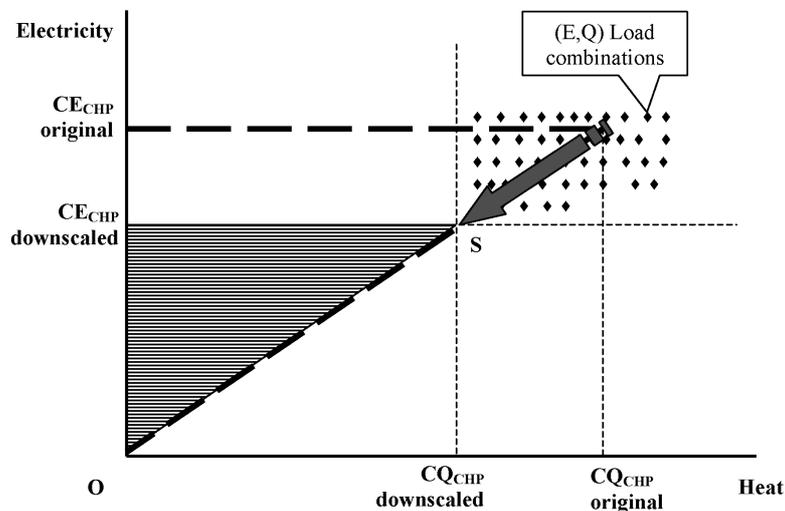
By reducing the dimension of the unit to a scale that guarantees a ‘certainty’ of useful heat all the time the unit is reduced in size. This is shown in Figure 4 by the downscaled  $CE_{\text{CHP}}$  and  $CQ_{\text{CHP}}$  values compared to the original ones. The downscaled plant will only meet part of the loads and it will have to buy make-up power at the grid and to consume fuels in the heat only boilers all the time to meet the load combinations.
