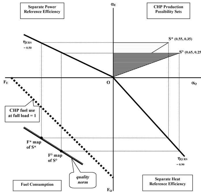
The conversion efficiency of a separate power generation reference process is added in the North Western quadrant and analogously for the separate heat reference boilers in the South Eastern quadrant (Figure 1). So doing one can finally compare in the South Western quadrant the fuel consumption of every  $(E, Q)$ -output pair that belongs to the CHP-feasibility set with the fuel consumption of the separate reference processes.
