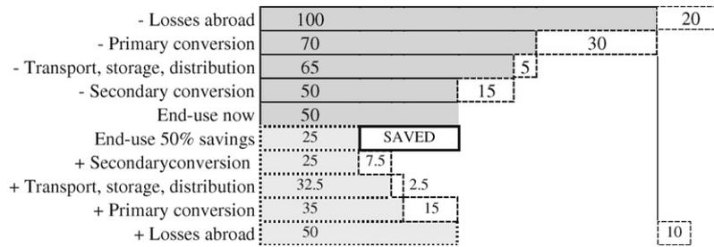
Fig. 5. Efficiency in end-uses is transmitted upstream in the energy supply chain.
