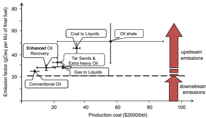
Fig. 1. Emission factors of liquid hydrocarbon resources, related to production costs (based on Brandt and Farrel, 2007).
