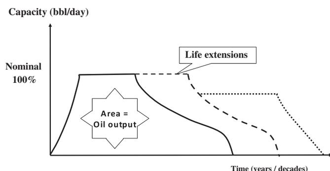
Fig. 3. Exploitation pattern of an oil deposit.
